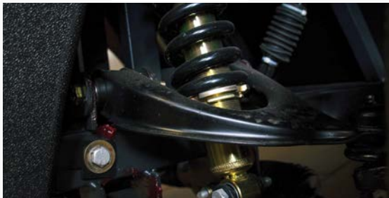
Independent suspension with double A-arms
