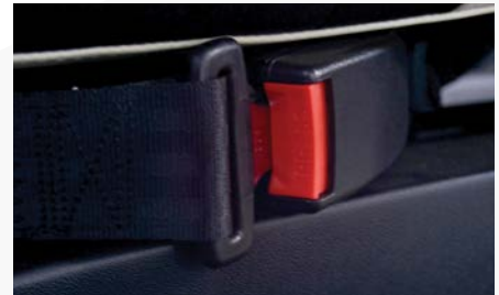
Type 1 or Type 2 seat belts conforming with 49 CFR § 571.209 – installed at each designated seating position.
