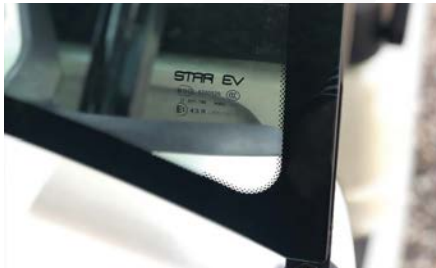
A windshield that conforms to the Federal Motor Vehicle Safety Standard (FMVSS) on glazing materials (49 CFR § 571.205).
